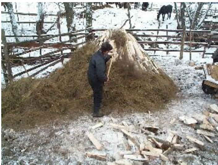
Shovelling down ash to cover the pile (This came from an old burning site) >>
