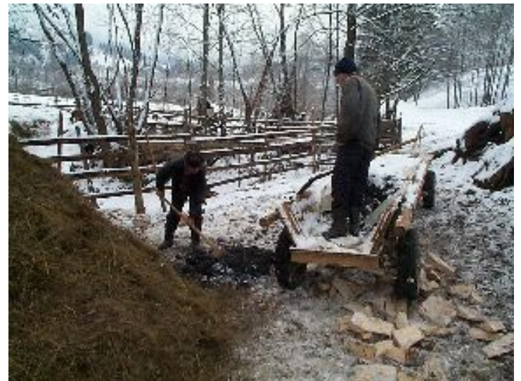
Shovelling down ash to cover the pile (This came from an old burning site) >>
